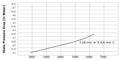
Air Flow (CFM) in 18" Diameter Duct
